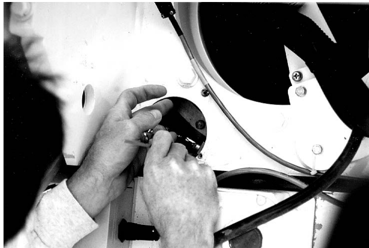
Figure 3. Adjusting Azimuth Cable Tension
