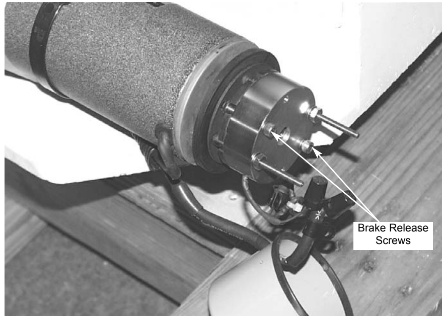
Figure 7. Brake Release Procedure. (azimuth gear motor shown, elevation gear motor similar)
