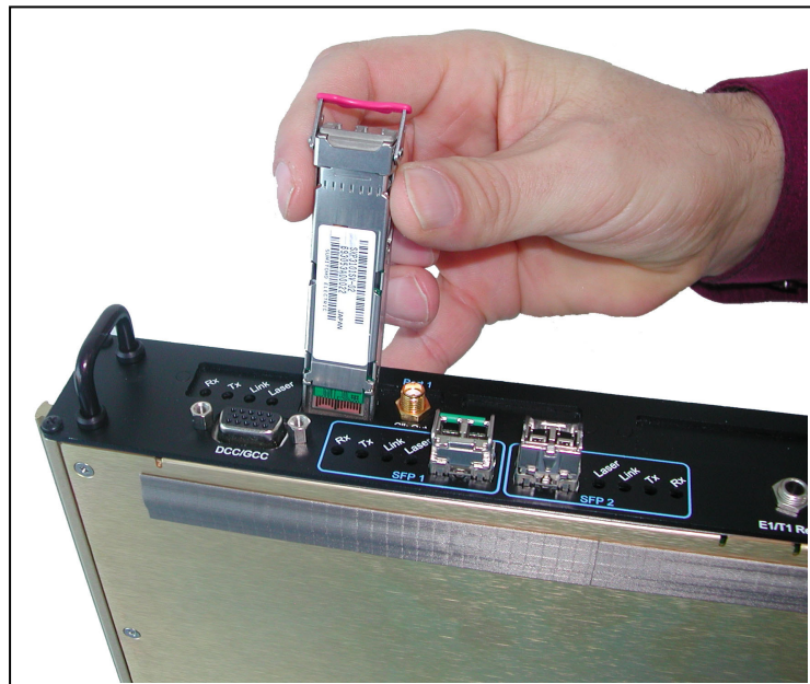
Fig.3: Change the optical interface of your module in the field via XFP/SFP transceiver
