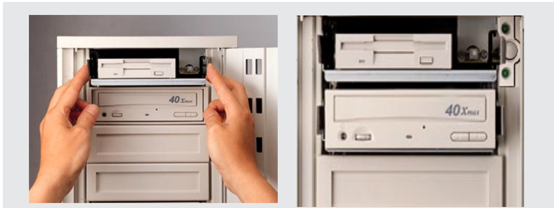
Removing a floppy or CD-ROM drive
