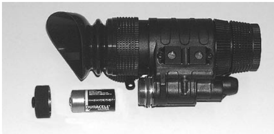
Figure 4-1 DL123 Battery Installation
