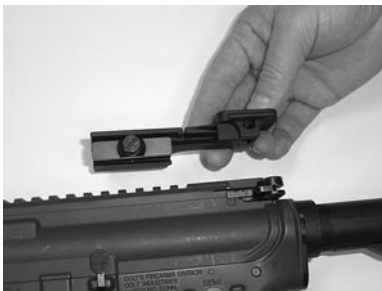
Figure 3-1 Attaching Weapon Mount to Weapon
