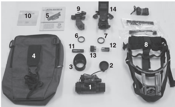
Figure 2-1 DNS ATN NVM-14 Major Components.
