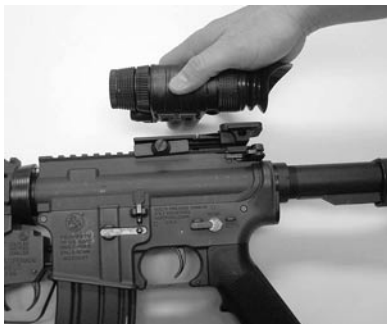
Figure 3-2 Attaching ATN NVM-14 to Weapon Mount
