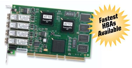
Quad-channel, 2-Gigabit Fibre Channel Connectivity, Featuring a PCI-X Interface, for High-performance Applications and Port Density
