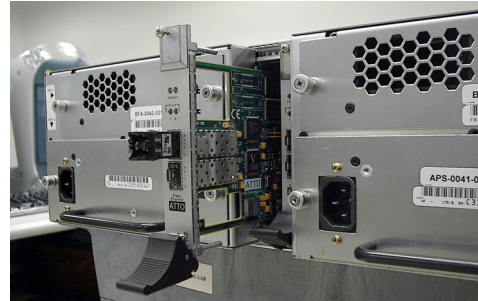
Exhibit 7-3: The Fibre Channel or SCSI Host Interface Card may be replaced by shutting power down, removing any cable attached to the port, removing the SFP according to manufacturer's instructions, loosening the screws at the top and bottom of the card, then carefully pulling out the unit.
