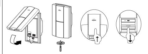
Switch all slave power bases to STANDBY by sliding the protective door upwards and positioning the switch to STANDBY.
