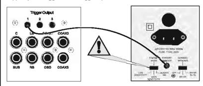
Plug the 8200X7 power cord into the mains supply. The amplifier will switch on briefly and then go to Standby. Switch the 8200AP on.
