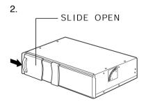
Insert the magazine firmly (which has been taken out of the unit) with the mark visible on the top side.
