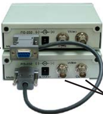
Figure 5F: Cable Connection to VSIB
