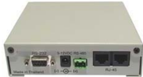
Figure 2H: Rear of TCPIP 232 Adapter
