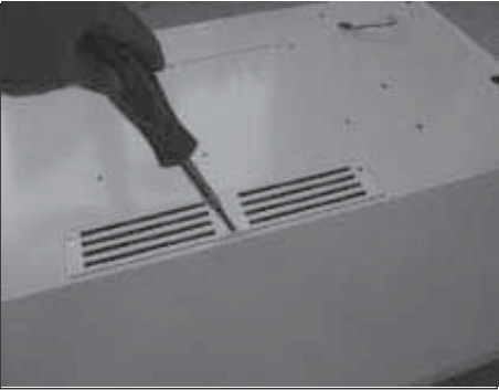
4. Remove the air recirculation louver plate on top of the hood.
