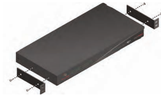
Figure 2.5: AMX Switch Rack Mounting Diagram
