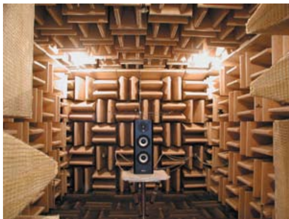
The M22ti being tested in the anechoic chamber at the National Research Center.
