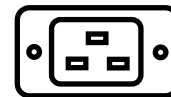
IEC 60320 C20 POWER INLET (9 amp) NOTE: Be sure unit is grounded. Check ground connection. Do not use if unit is not grounded.
