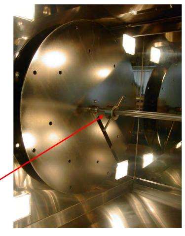
To remove the discs from the central shaft, simply unscrew the retaining nut that releases the disc for removal.
