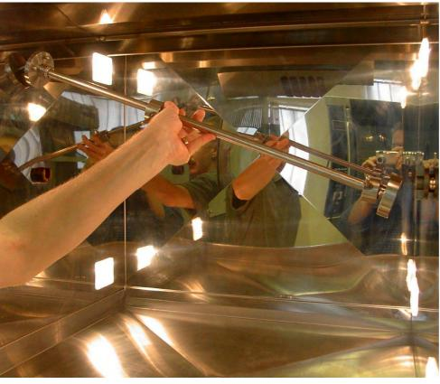
Remove the central shaft by lifting and withdrawing from the drive coupling.
