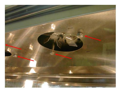
To remove an element cover, unscrew the four retaining nuts.
