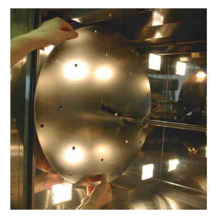
To remove the discs, withdraw from the drive pins and slide off the shaft, the shaft passing through the slot provided.
