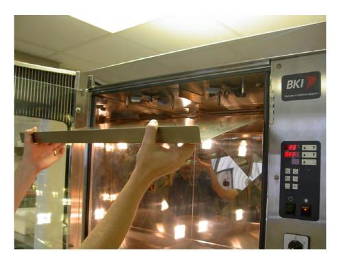
... And slide the cover out from the oven cavity.
