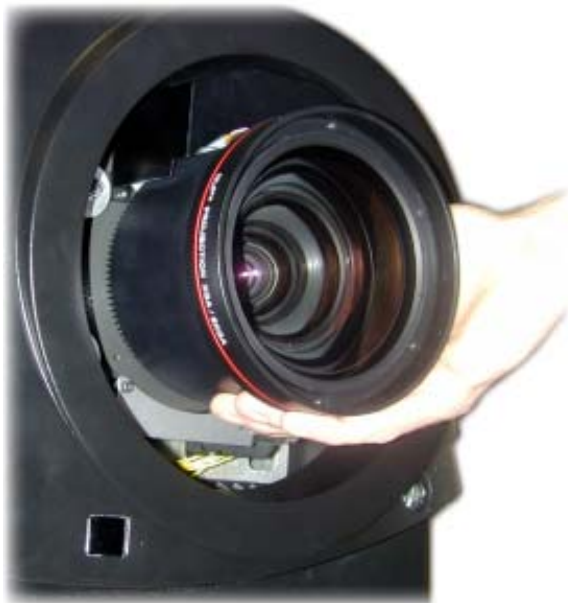
Image 1-1 Support the lens with one hand
