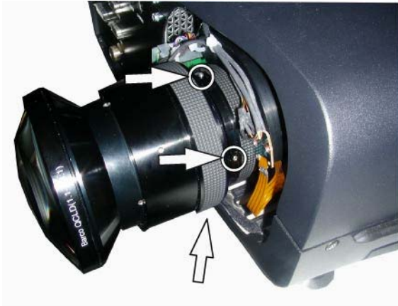
Image 2-6 Tighten the fixation screws of zoom ring
