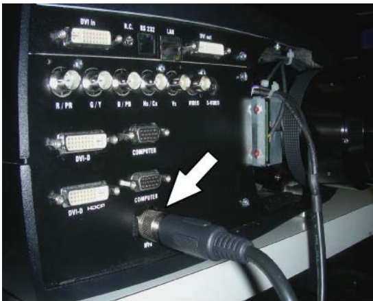
Image 2-7 Connect the wire from the lens to the NVG input
