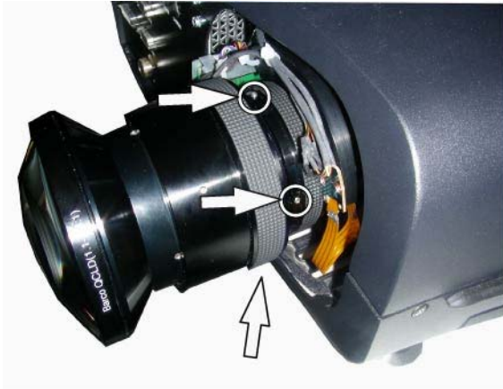
Image 2-2 Screws to loosen the zoom ring
