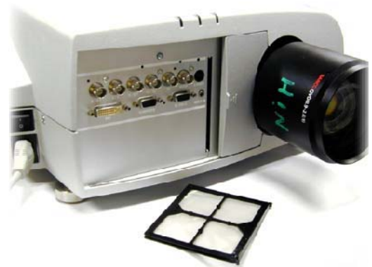
Image A-6 Input filter removed
