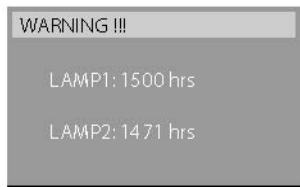
Image 4-8 warning message in case of a IQ300 series projector
