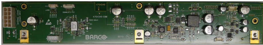
Figure 15: Front view of the Power Interface Board
