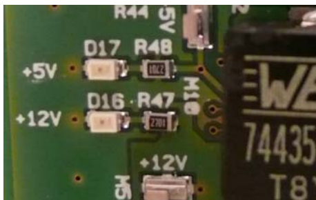
Figure 16: Indicator LEDs on the Power Interface Board
