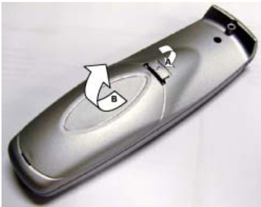
Image 3-3 Battery cover unlock
