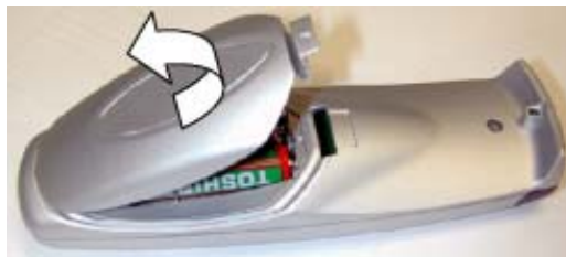
Image 3-4 Battery cover removal
