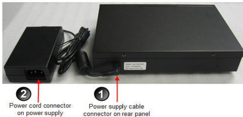
Figure 23 Attaching the power cables on the ET0010A-402
