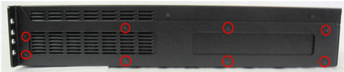
Figure 37 Each bracket is attached to the side of the ET10000A using eight screws
