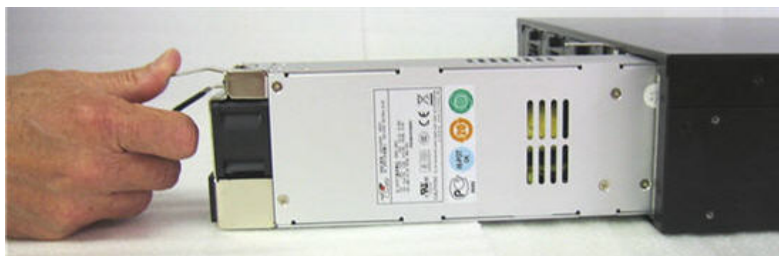
Figure 48 Remove the power supply from the chassis
