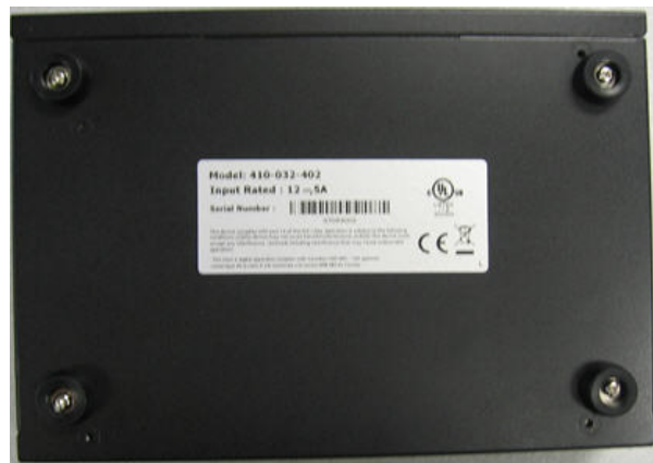
Figure 20 Rubber feet installed
