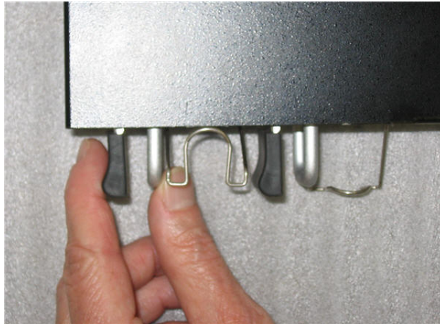
Figure 44 Release lever on power supply # 2
