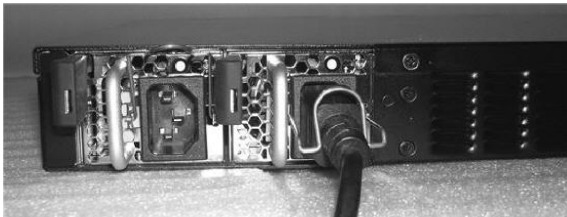
Figure 34 The power cord for power supply # 1 is secured with a clip
