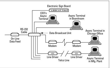
Enhance a security system with parallel data output using the Parallel Data Broadcast/Fallback Unit.
