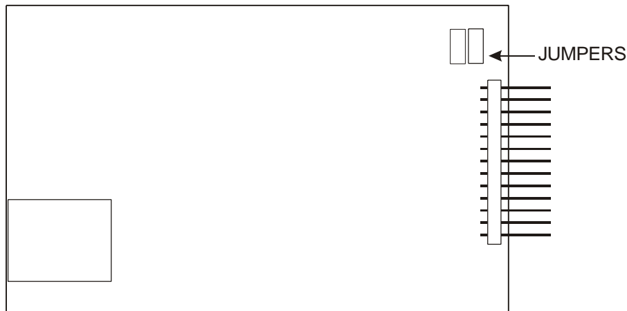
Figure C-4 ISDN Module processor setting jumpers
