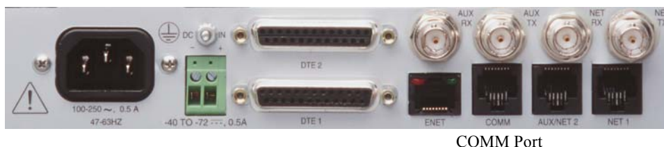
Figure 3-2 COMM Port on Dual Trunk E1 Router
