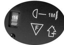
Figure 1 - AC Voltage Switch
