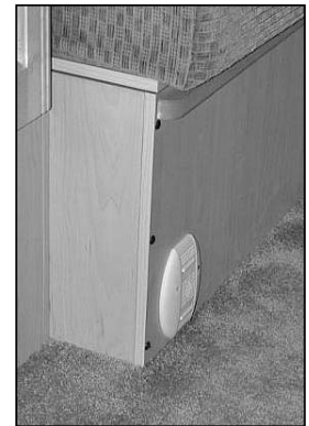
Picture F-P1A: L.P.G. leak detector, Versatile model.
