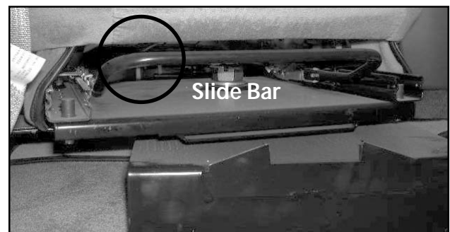
Picture B-P1A: View of the front of the Captain's seat, showing the location of the slide bar.
