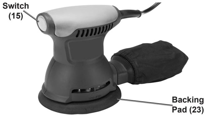
The Sanding Disc is attached by Hook and Loop to the Backing Pad. Place the Sanding Disc on the Backing Pad lining up the 8 holes so that the dust can be collected into the Dust Bag.
