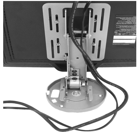
Figure 7. Route Cables Down Arm
