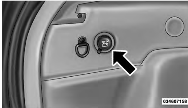
Rear Power Outlet
