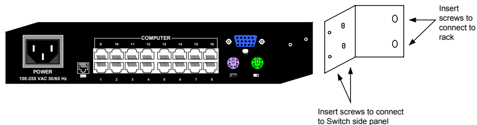
Figure 7 Connecting the L-shaped bracket
