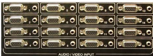
Figure 2 - Audio and video inputs on AC1123A
