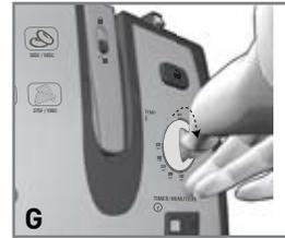
1. Select the desired cooking temperature by turning the temperature dial so that the point on the dial is directly at the desired temperature (G).
