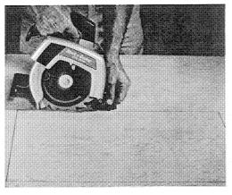
allow blade to stop completely before withdrawing the blade from the material. When starting each new cut, repeat as above. Never tie the blade guard in a raised position.
