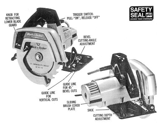
**CUTTING DEPTH:** At  $90^{\circ} - \frac{1}{8}$ " to  $2\frac{3}{8}$ ". At  $45^{\circ}$  bevel -0" to  $1\frac{3}{4}$ ". BEVEL ADJUSTMENT: 0° to 45°.
