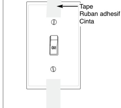
• Note whether the light turns on when the switch is flipped up, or when the switch is flipped down. The Auto Switch can be configured for either case.
