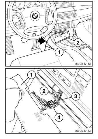
Connect other end of extension wire (2) to violet/blue wire (3) located in pin location 23 of switching center (1) connector X1869 using quick connector 61 13 8 364 566 (4).
