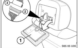
Using special tool 00 9 340 (1) pry monitor
