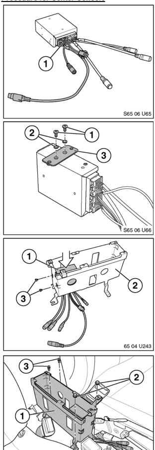
1. Insert white A/V connector (1) P/N 84 11 0 399 309 into A/V module as shown.
