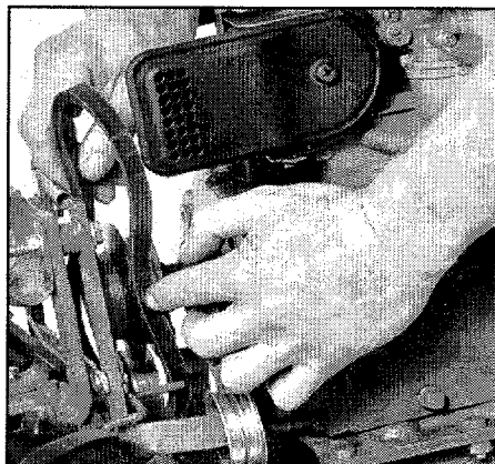
Figure 5-18: Install forward drive belt over rear of engine forward pulley and bring lower half of belt down and in front of transmission pulley.
