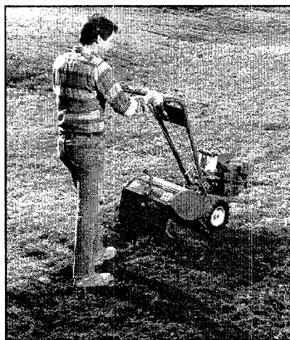
Figure 4-4: To begin turn, reduce engine speed and lift handlebars until engine and tines are balanced over wheels.
