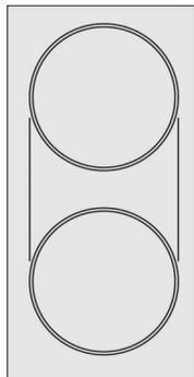
The bridge element connects two separate elements to create one long element. This shape is ideal for griddles or roasters.
