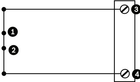
Figure 9.3 N.C. Normally Closed Connections
