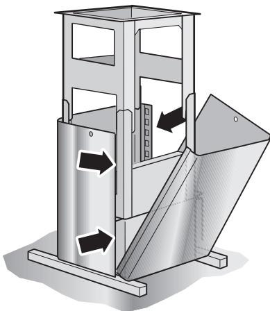
15. Push up the upper flue section and screw into position.
