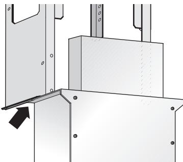
9. Screw the extractor hood to the support frame and screw back the panel.
