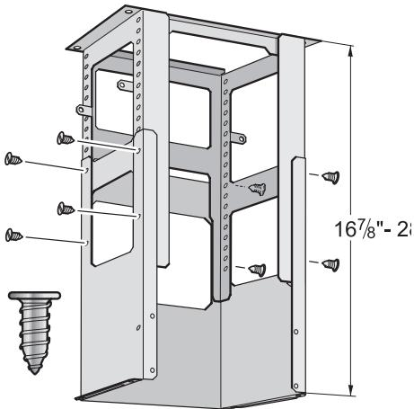
6. Screw the support frame to the ceiling with 4 screws.
