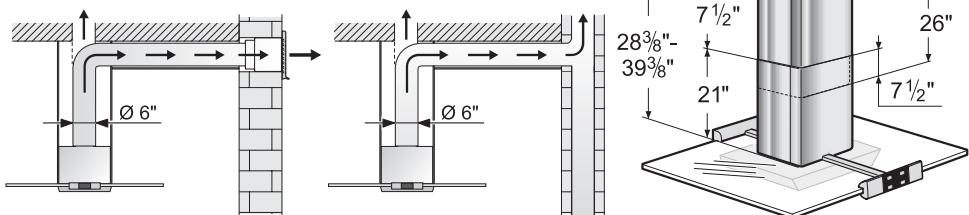
The exhaust air is discharged upwards through a ventilation shaft or directly through the outside wall into the open.
