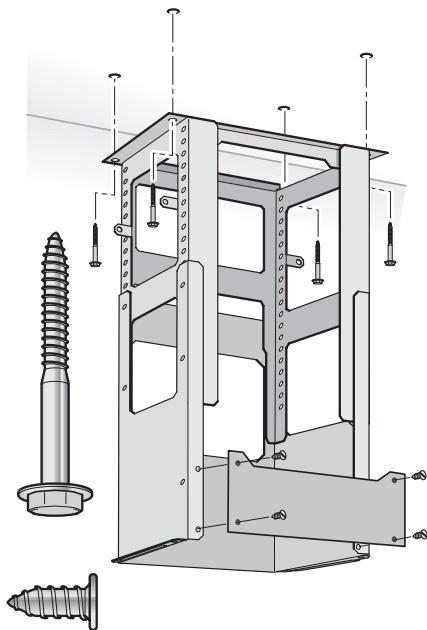
8. Insert the extractor hood over the installation aids on the support frame.
