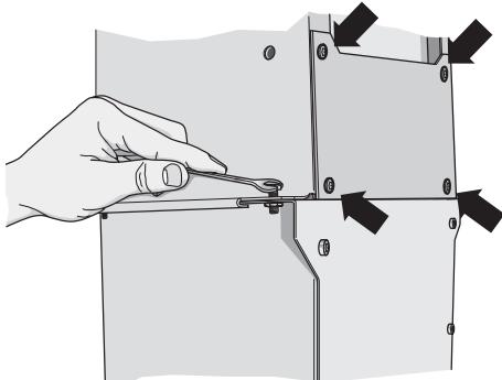
10. Align the extractor hood. To do this, loosen the ceiling screws in the support frame.
