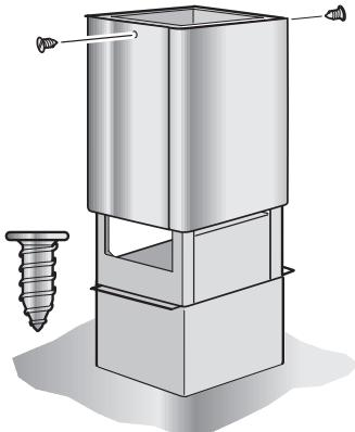
16. Insert the two sections of the lower flue and clip together.
