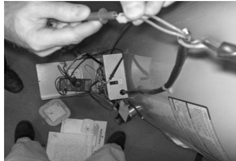
Checking continuity of upper sensor wire harness.
