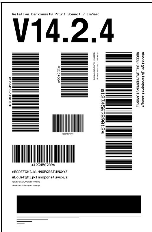
Figure 3.4 Feed Key Test Sample Printout
