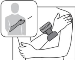
5. The positioning system (A) shown on the left and a beep confirm that you have reached the right measuring position. The measurement will start automatically. When the measurement is complete, a beep will sound again, and the reading is displayed:
