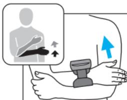
1. Place the monitor housing on the slim side of your bare forearm with the monitor facing up. The distance aid (H) helps you to keep the required 2 cm distance to your palm line.
