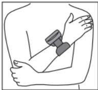
For accurate measurements, all wrist blood pressure monitors must be positioned at heart level. Example: If the monitor is positioned 20 cm below heart level as shown on the left (e.g. by putting the arm on a table), the reading you will obtain is approximately 15 mmHg too high.
