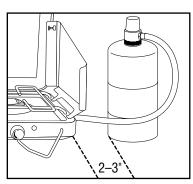
**NOTE:** Propane canister should be positioned a minimum of 2–3" from stove. Always use a canister with a flat bottom.
