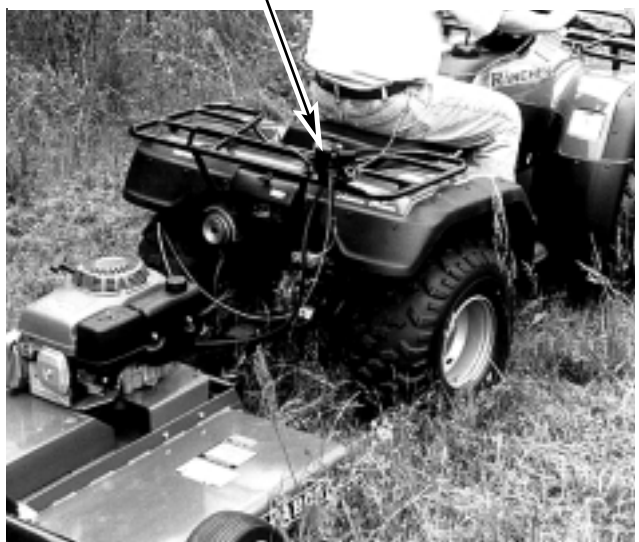
Figure 2-4 Control Box Mounted On ATV Rack
