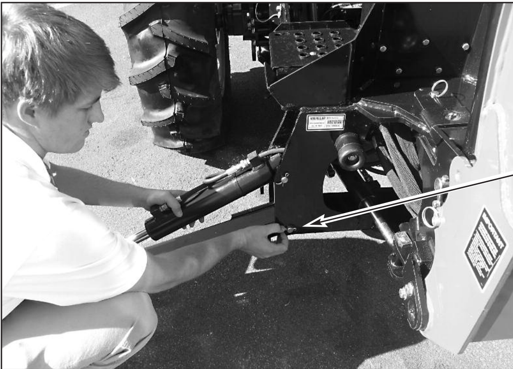
Pinning Stabilizer Into Place
