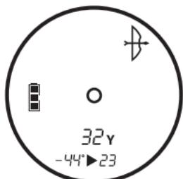
When line of sight distances from 5-99 yards are displayed, the Bow mode indicator will automatically be displayed along with angle and a compensated distance. If distances greater than 99 yards are displayed, the Bow mode Indicator will automatically turn off along with compensated distances.
