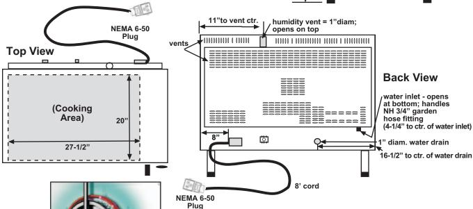
**Steam:** Water is injected directly into the baking chamber, vaporized and changed into steam when touching the hot heating element. Water should be connected to the oven water inlet by a mechanical filter and a cut-off valve. Water must have a hardness between 0.5°-5°F in order to reduce formation of limestone deposits inside the electro-valve and inside the cooking chamber, and a pressure value between 0.5 - 2 bar (7.25 - 29 PSI.)
