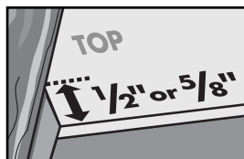
FIGURE 3 Face of wall can must extend ½ inch or 5/8 inch from face of stud to allow for thickness of sheetrock. Mount wall can flush with finished surface.
