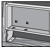
FIGURE 1 Metal legs position wall can at minimum floor clearance.
