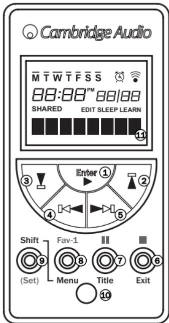
Buttons numbered 1-8 have dual functions, which are controlled by the *Shift* button. These buttons generate IR codes or macros cloned from the buttons of the same name on the LR10 learning remote (see later section on Cloning).
