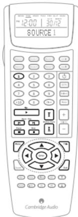
For the LK10 to receive commands, it must be first put into Learn mode. The LK10 has a series of menus that can be accessed by pressing and holding the *Shift/Set* button on the front panel. The menu options are continuously scrolled on the LK10 display until you release the *Shift/Set* button.
