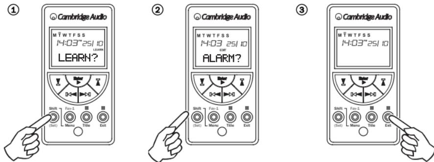
To select the option you require release the button when the menu option is displayed on the screen (Fig. 2).
