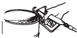
Figure 4 - Spray Gun Against Metal Container
